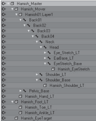
Figure 3.6-6. Final hierarchy of ItemID. To change the display order to ItemID, click in the Name bar above the item display.
