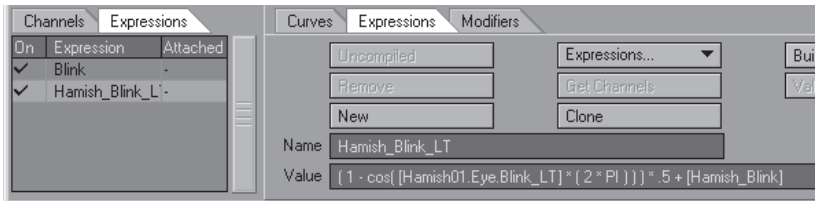
Figure 4.2-13. [Hamish_Blink] references the Blink expression. Adding [Hamish_Blink] to the expression means the helper morph will work for the left eye blink morph as well as the combined blink morph.
