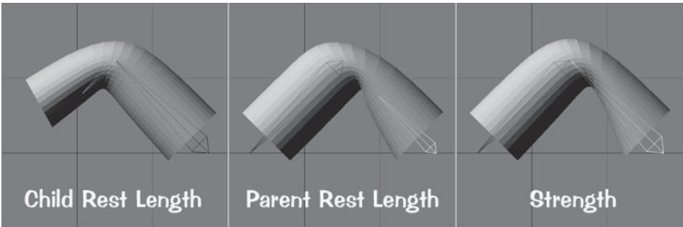
Figure 3.8-4. Bones sharing a weight map. Notice that changing the rest length produces a different result than just changing the strength.
